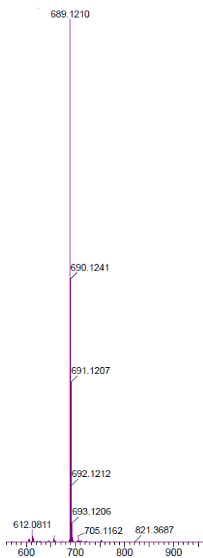
Figure 14 MALDI TOF/TOF mass spectrum of III.6 (Calculated mass for C_{42}H_{28}N_2S_4 is 688.1135).
