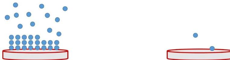
*Figure 4 Schematic of analyte-sorbent interface at ambient and ultrahigh vacuum conditions respectively. (www.orsayphysics.com)*
