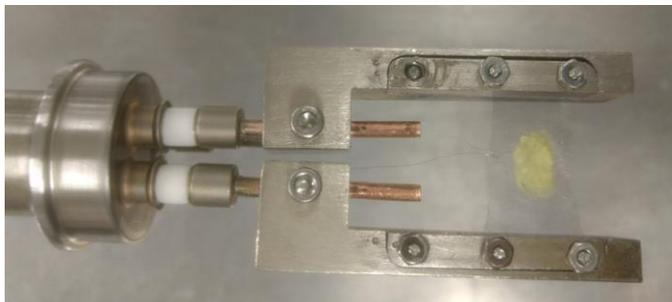
*Figure 11 Sample manipulator with DC-4 coated on the tungsten mesh*
