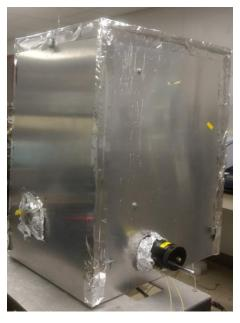
Figure 12 Image of bakeout of a vacuum chamber using reflective plates and heating tapes (not seen in the image)
