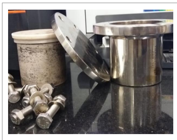
Figure 2.3 Autoclave for hydrothermal synthesis of nanomaterials.
