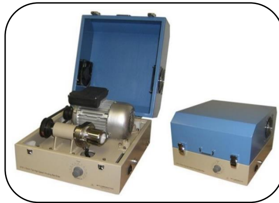
Figure 2.9 Ball miller instrument.
