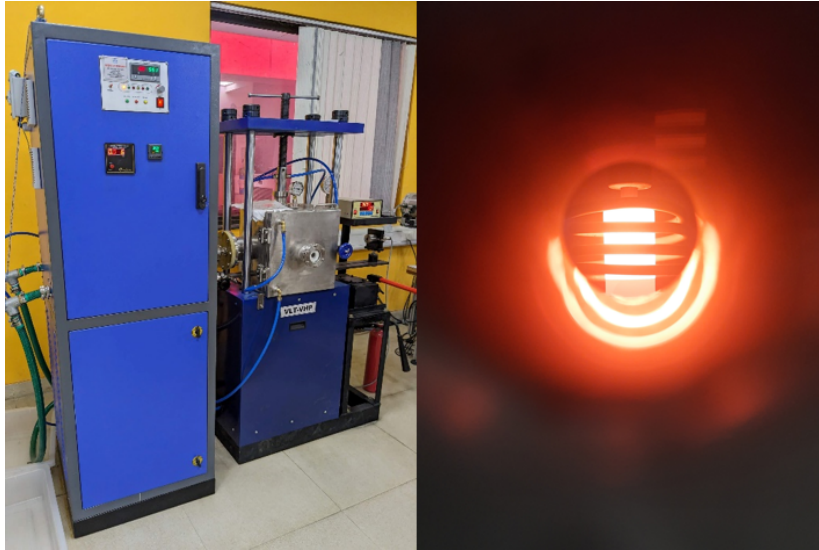
Figure 3.3: Hot Press (let), Heating coils and graphite die inside the chamber (right).
