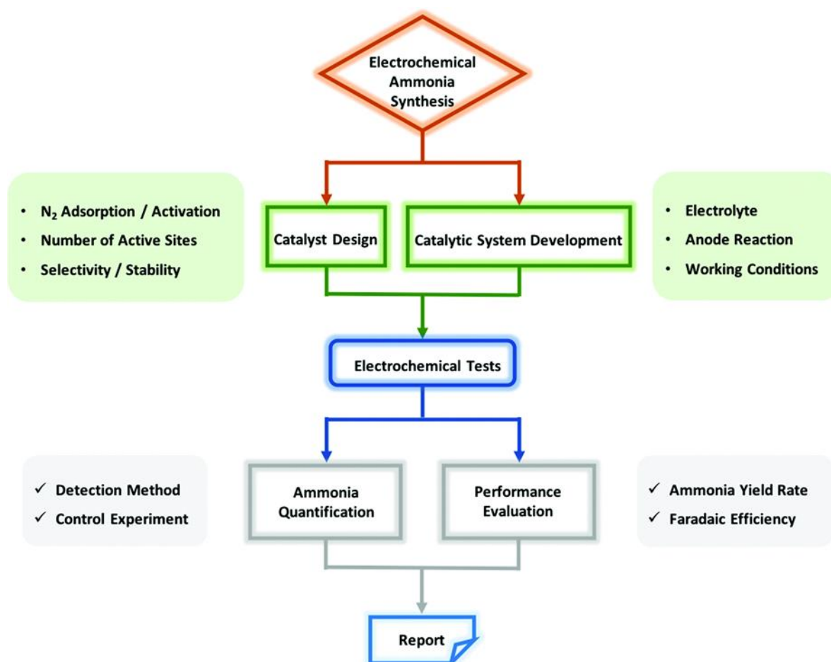
Figure 1.25: A Flowchart for electrochemical NH 3 synthesis. (Adopted from Ref 112)
