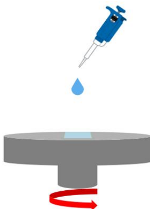
Fig 2.6: Schematic representation of Spin-coating [45]
