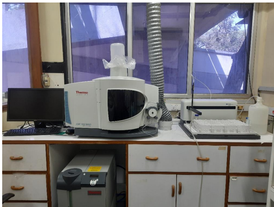
Figure 2.8: ICP-OES at PRL, Ahmedabad
