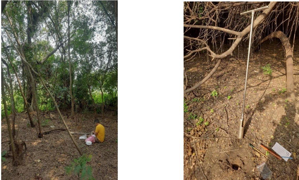
Figure 2.3: Sampling site (left) and the corer used for sampling (right)
