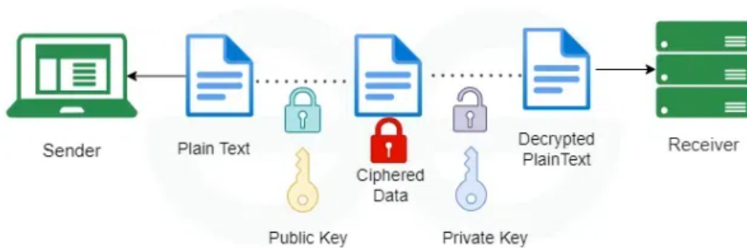
Figure 2.2: Public Key Encryption Process: The sender encrypts the plaintext using the recipient's public key, and only the recipient can decrypt it using their private key.
